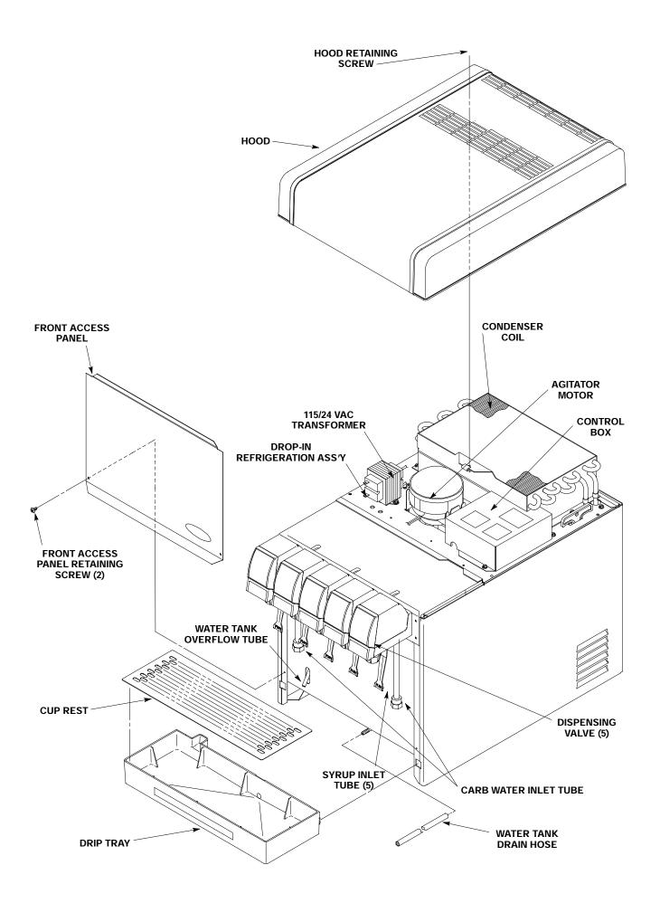
2. Check the dispensing valves for dripping that indicates leakage and repair as necessary.
